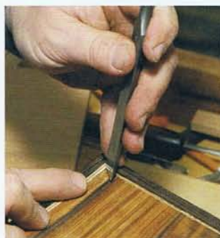
PRESS THE INLAY INTO THE GROOVE WITH THE BACK OF A CHISEL (left). It should not need clamping or taping. Fine-tune the miter if necessary (above).
