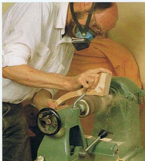
SANDING ALL THE LEGS TO THE SAME SHAPE is easier if the blanks are taped together before sanding to the layout lines. Bandsawing the legs close to the line reduces sanding.
