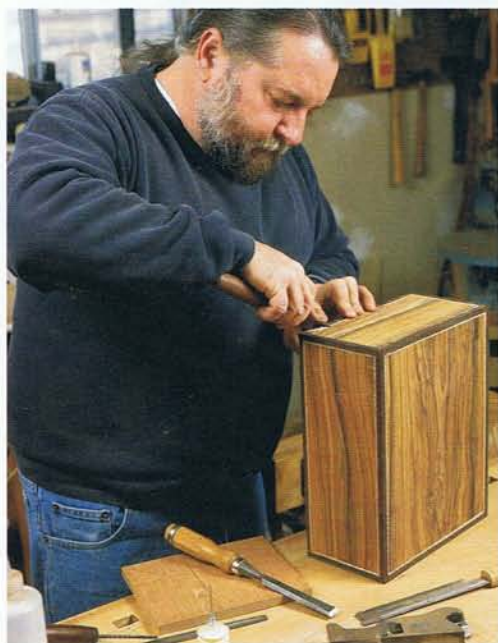
PRESS THE INLAY INTO THE GROOVE WITH THE BACK OF A CHISEL (left). It should not need clamping or taping. Fine-tune the miter if necessary (above).
