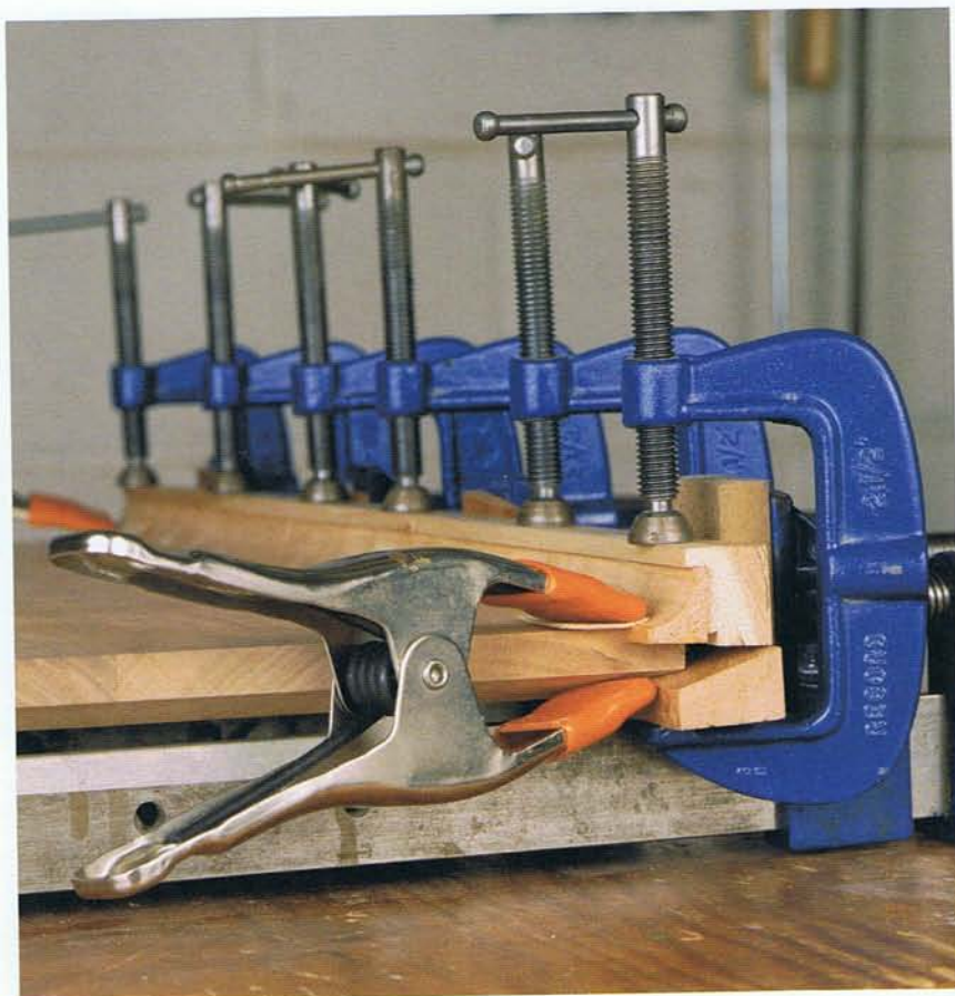
RABBETED CLAMPING BLOCK HELPS PROVIDE PRESSURE IN TWO PLANES. The author clamps down the cove strip with six C-clamps and into the rabbet with six bar clamps. A spring clamp on each end closes any visible gaps at the ends.
