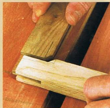
A PERFECT FIT. It's best to work out any problems before you begin glue-up. A dry run ensures that everything fits and that the bridle joints pull tight.
