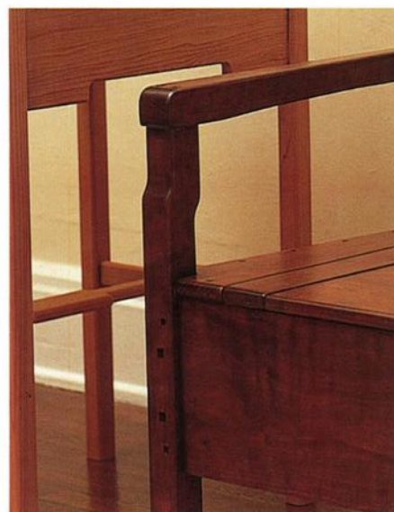
The Greene brothers were U.S. designers and builders who worked in the early 1900s. Their pieces included Japanese design elements. The stepback at the top of the front leg on this bench is a good example of the subtle but effective design elements they used.
