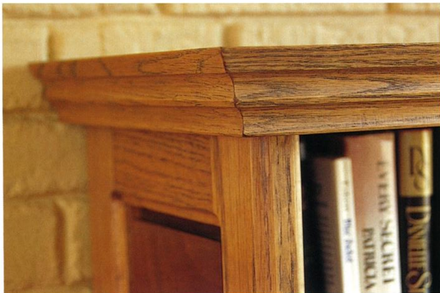
This simple crown moulding is made by cutting two parallel grooves in the top moulding strips. The same core-box bit used elsewhere on this bookcase was used to create these grooves.
