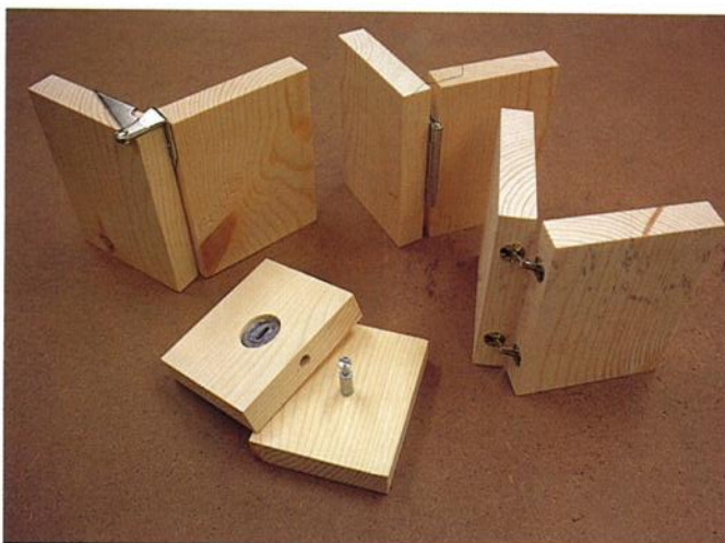
This is hinge hardware in action. Clockwise from the upper left: pivot hinge, butt hinge, hidden hinges and a set of knockdown hardware.
