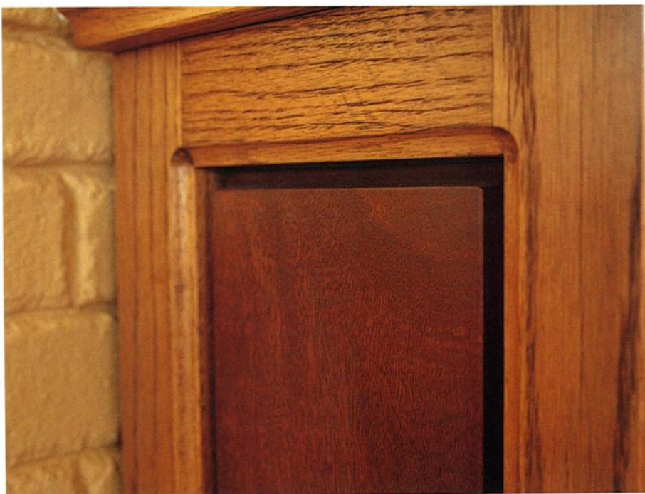
These sides have raised panels made with a core-box router bit. That same bit is used to rout a cove on the inside edges of the side's frame.
