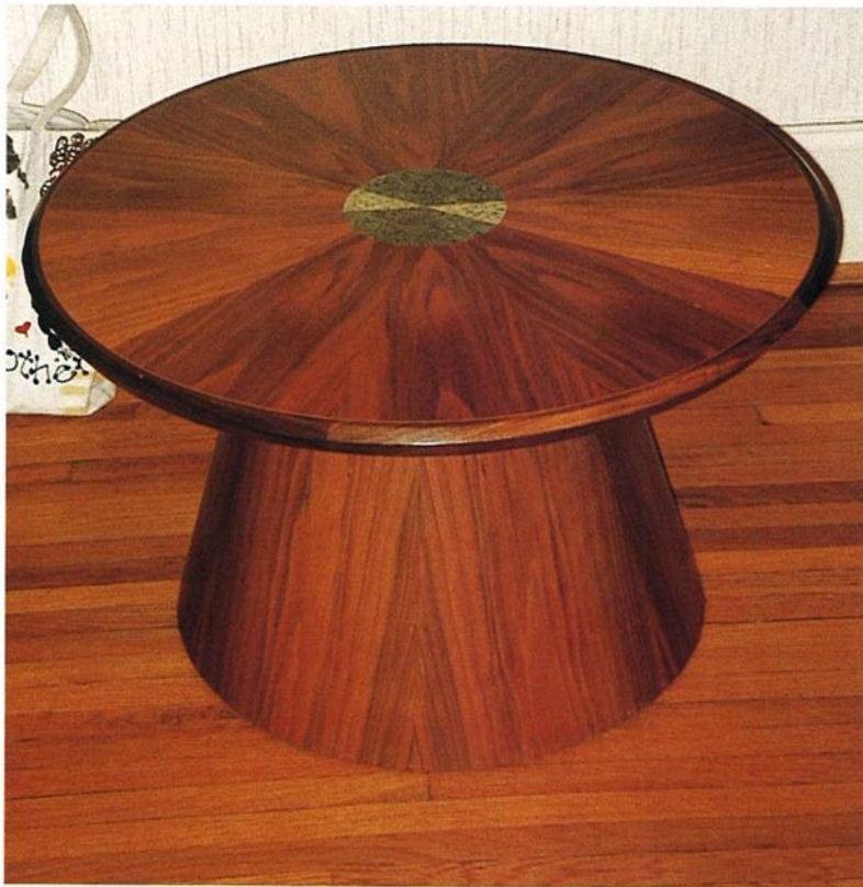
Walnut veneer was used in a starburst pattern to create the design for this coffee table. The pattern is bookmatched on the top and the cone base. Getting the veneer to match and wrap around the base was a great challenge! The results exceeded my expectations.
