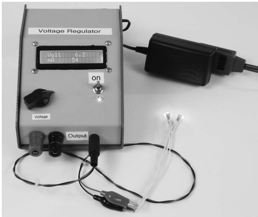
Figure 3-9: The completed Regulated Power Supply
