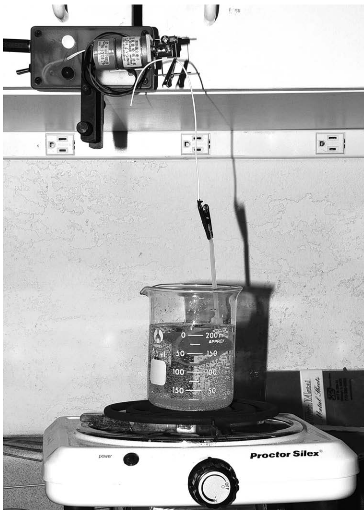
Figure 2-22: This Arduino-based etcher-agitator etches a board. The etchant should turn emerald as the copper is etched. The board is held by a wire tie that is attached to a wire by an alligator clip. The wire goes through a hole on the crank and is held in place with another alligator clip. One of the LEDs is lit.
