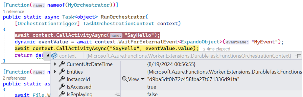
Figure 7.4 – IsReplaying is false
