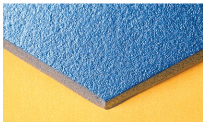
Two layers of Flexbond for Worbla were applied to this sample before painting.
