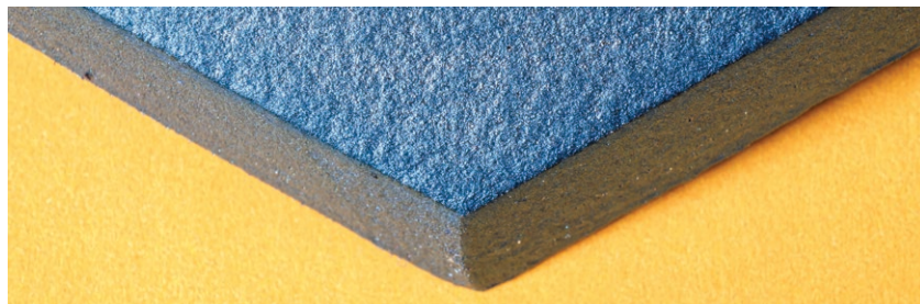
Two thin layers of Rapid Fill were applied and lightly sanded to reduce brushstrokes.
