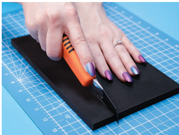
The blade is perfectly perpendicular to the cutting mat.
