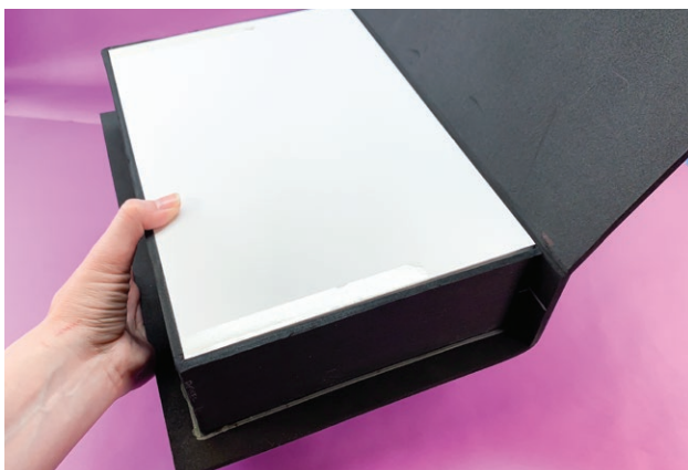
10. Use a strong double-sided adhesive tape like CosBond to tack the box top to the cover. Place strips of tape along the edges of the foam core.
