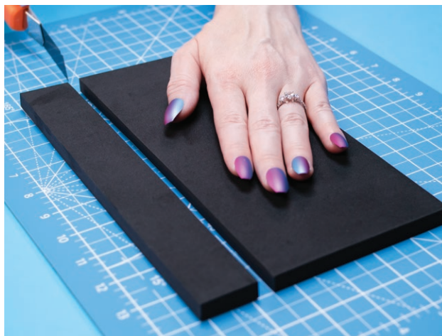
The blade is perfectly perpendicular to the cutting mat.
