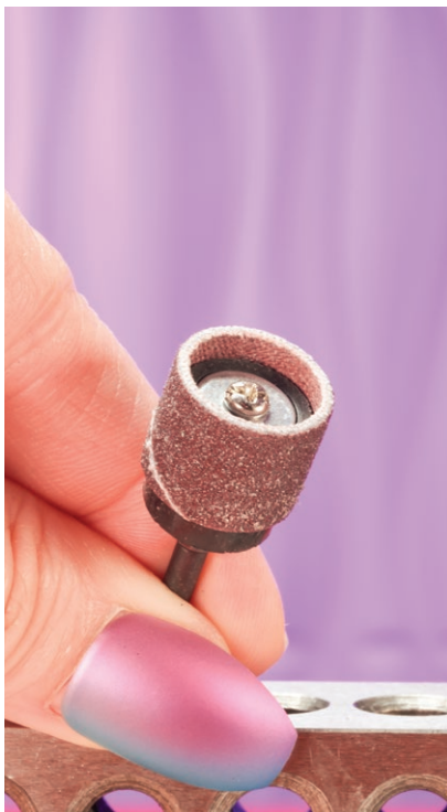
2. Offset the barrel to the desired depth and retighten the screw.
