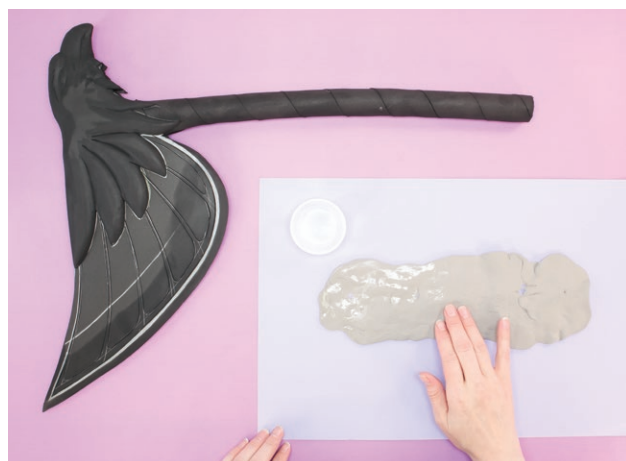
Apply water to the foam clay and the EVA foam for better adhesion, as I did when making this Eagle Axe designed by Mathew Grigsby.
