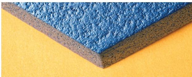
Three layers of Krylon Fusion All-In-One were applied to this sample before painting.
