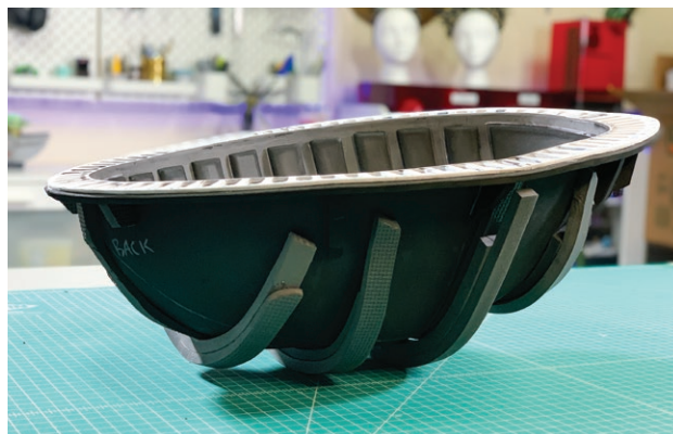
The hollow shell of this pod prop was reinforced by adding several strips of scrap EVA foam to create an inner support structure.
