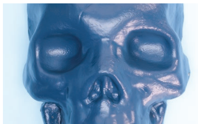
This thermoplastic skull was created by forming MTP over a skull shape, creating a smooth surface.
