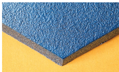
Three layers of Plasti Dip were applied before painting.
