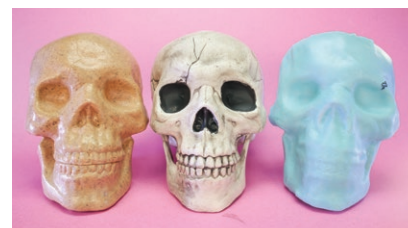
This skull decoration ( center ) was used to create two thermoplastic shells: the shell on the left from smooth MTP and the shell on the right from reinforced Thibra Tex.
