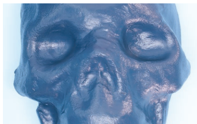
This thermoplastic skull was created by forming Thibra Tex over a skull shape, creating a very strong shell with a textured surface.
